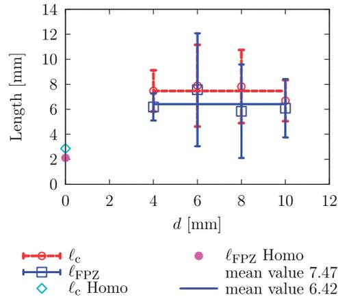
**Figure 21.** Variation of the characteristic length of the material  $l_c$  and the FPZ size  $l_{FPZ}$  with respect to the inclusion size  $d$  within the path ② of variation.
