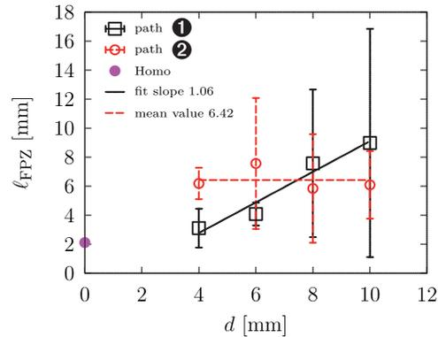
**Figure 9.** Relation between the FPZ size  $\ell_{FPZ}$  and inclusion size  $d$  with respect to the variation paths ① and ② ( $3\phi$ ).
