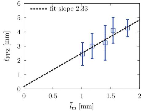
**Figure 4.** Evaluation of the FPZ size (4 standard deviations of statistical distribution of energy releases on either side of the average crack path) with respect to mesh size: the FPZ size  $\ell_{FPZ}$  does statistically vanish under mesh refinement.
