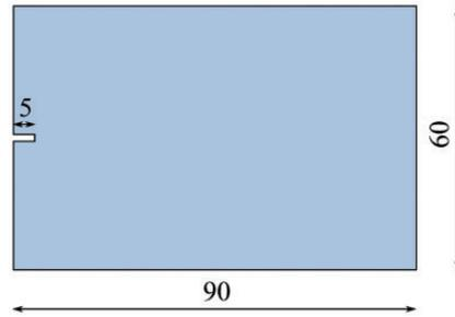
**Figure 13.** Specimen dimensions [mm].
