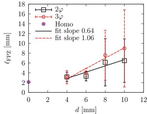
**Figure 7.** Affine relationship between the width of FPZ  $\ell_{\text{FPZ}}$  and the diameter  $d$  of the inclusions, with (3 $\varphi$ ) or without (2 $\varphi$ ) weak interfacial transition zone between inclusions and matrix is observed using the variation path ①.
