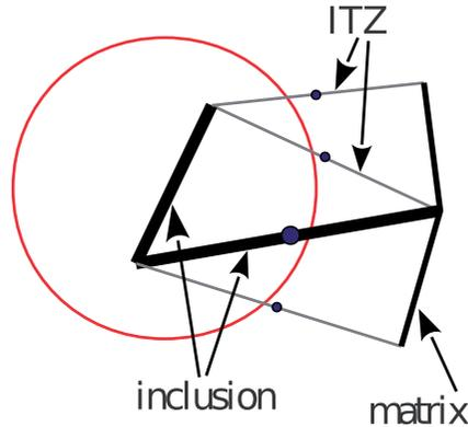
**Figure 2.** Distinction between inclusion, matrix and ITZ phases according to the location of a lattice element in the grain structure.
