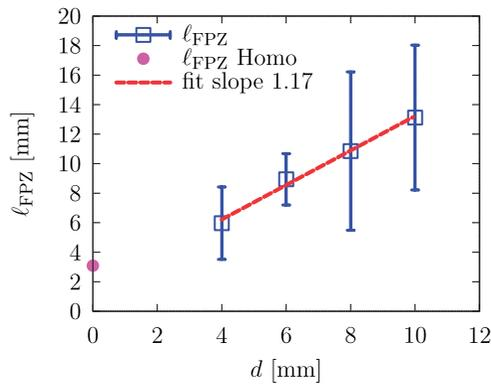
**Figure 14.** Variation of  $l_{FPZ}$  according to the inclusion size  $d$  of the variation path ①, obtained from tests with specimen dimensions shown in Figure 13.
