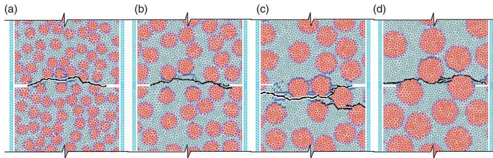
**Figure 10.** Crack patterns and the corresponding FPZ size  $\ell_{FPZ}$  [mm] of the LD tensile tests on the specimen made of the material with different inclusion constant-size  $d$  [mm] of the variation path ② ( $P_a$  ranging from 30% to 40%). Blue and black points are the broken elements: black for wide-open macro-cracks and blue for barely-open micro-cracks. The sample dimensions are shown in Figure 3a. The mean number of elements per macro crack is in the order of 80.
