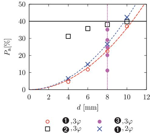
**Figure 5.** Three variation paths ①, ② and ③ for three-phase material (3φ) and the variation path ① for two-phase material (2φ) in the ( $P_a \leftrightarrow d$ ) parameter space for the monodisperse distribution of inclusions.
