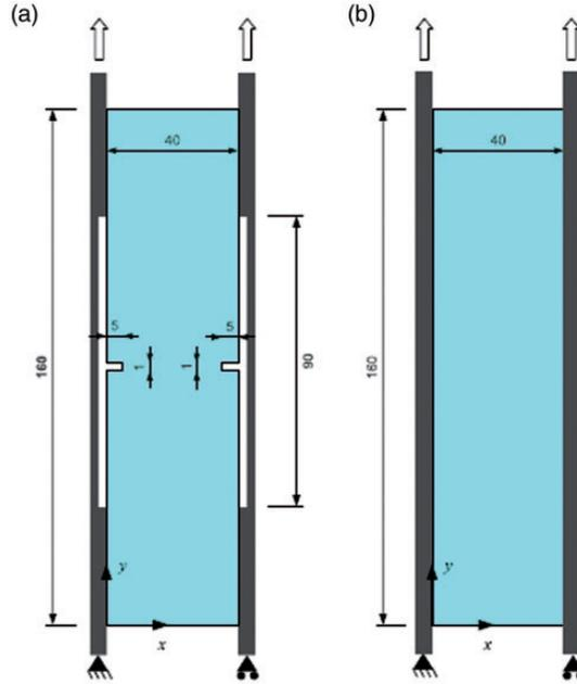
**Figure 3.** Sketch of the specimens used to determine the characteristic length as proposed by Bažant and Pijaudier-Cabot (1989). The tensile test performed on the notched specimen to obtain the localised cracking process (a) and on the non-notched specimen to obtain a distributed cracking process (b).
