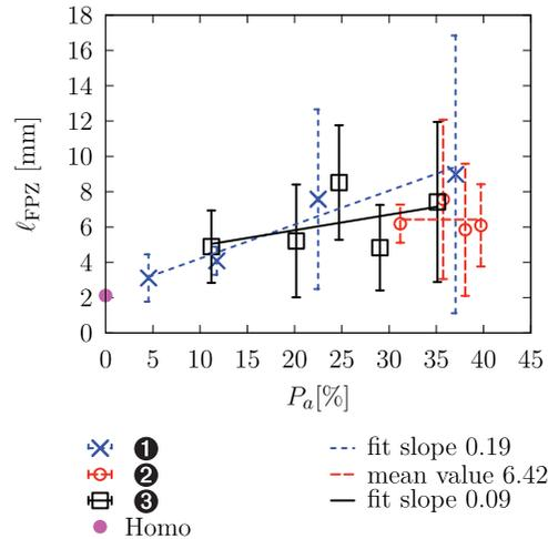
**Figure 12.** Variation of  $l_{FPZ}$  according to the inclusion surface fraction  $P_a$  of the three variation paths ①, ② and ③. The sample dimensions are shown in Figure 3(a).
