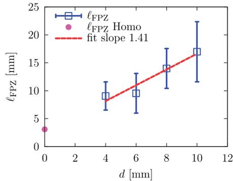
**Figure 15.** Variation of  $l_{FPZ}$  according to the inclusion size  $d$  of the variation path ② (with specimen of Figure 13).
