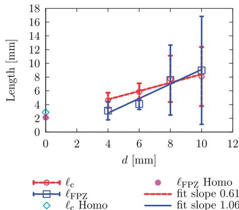
**Figure 20.** Variation of the characteristic length of the material  $\ell_c$  and the FPZ size  $\ell_{\text{FPZ}}$  with respect to the inclusion size  $d$  within the path ① of variation.
