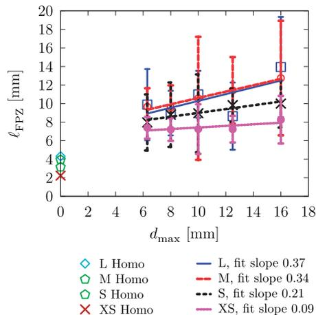
**Figure 18.** Influence of the ligament length on the variation of the FPZ size  $l_{FPZ}$  with respect to the maximum inclusion size  $d_{\max}$ : L (long ligament), M (medium ligament), S (small ligament), XS (extra small ligament).
