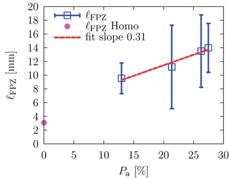
**Figure 16.** Variation of  $l_{FPZ}$  according to the inclusion surface fraction  $P_a$  of the variation path ③ (with specimen of Figure 13).
