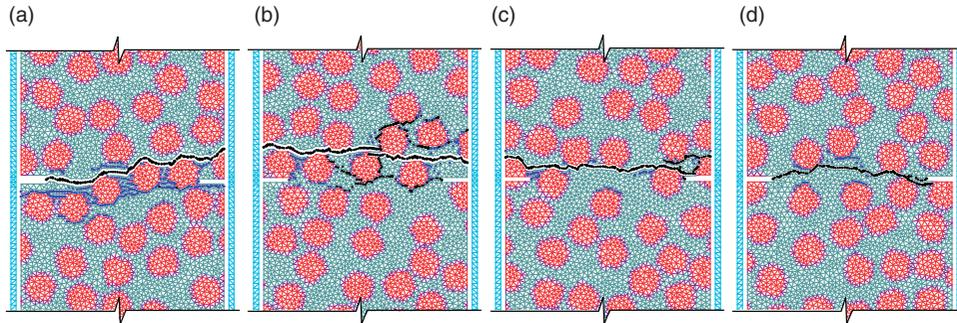
**Figure 11.** Crack patterns and the corresponding FPZ size  $\ell_{FPZ}$  [mm] of the LD tensile tests on the specimen made of the material with inclusion size  $d = 6$  mm with four different position distributions of the inclusions ( $P_a \simeq 35\%$ ). Blue and black points are the broken elements: black for wide-open macro-cracks and blue for barely-open micro-cracks. The sample dimensions are shown in Figure 3(a). The mean number of elements per macro crack is in the order of 80.
